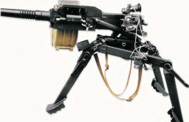
AGS 17 an Automatic Mounted Grenade Launcher
